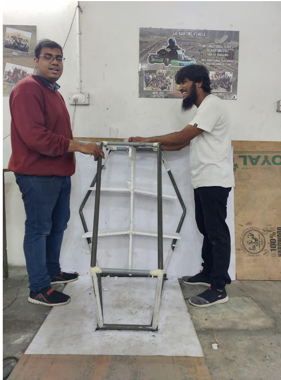
Roll cage with PVC supports
